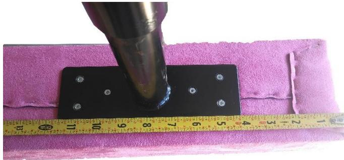
3. Install all the 6 screws tight. The center of the riser is about 8" from the edge.
